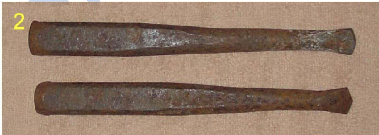
Typical Plug Drills - (Top) drill with a round blade (bottom) drill with pointed blade
