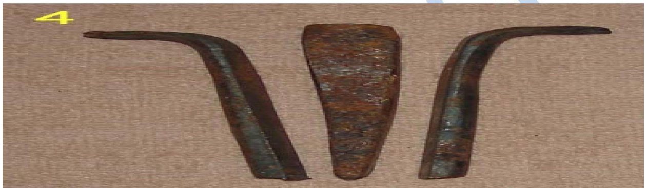
Two feathers (shims) with a plug (wedge) between them
